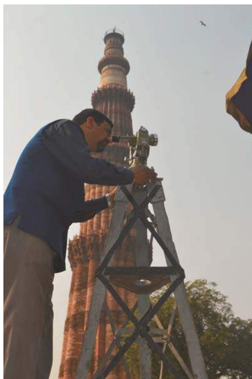
Observations for checking the verticality of Qutub Minar
