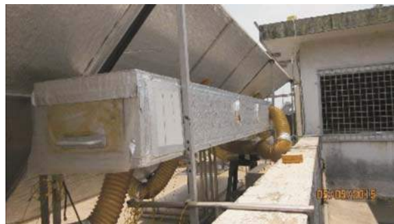
Various Solar Air Heaters Developed at HPL_IITB Integrated with Drying Duct for Preliminary Testing
