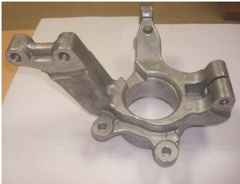
Fig. 3. Machined rheo pressure die cast steering knuckle
