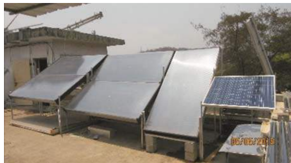
Various Solar Air Heaters Developed at HPL_IITB Integrated with Drying Duct for Preliminary Testing
