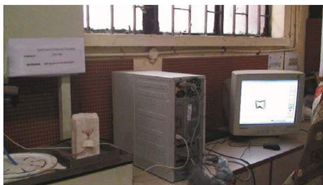
Instrumental set-up for the in-plane wicking
