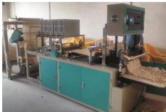
Machinery set-up for converting nonwoven fabric into fruit bags
