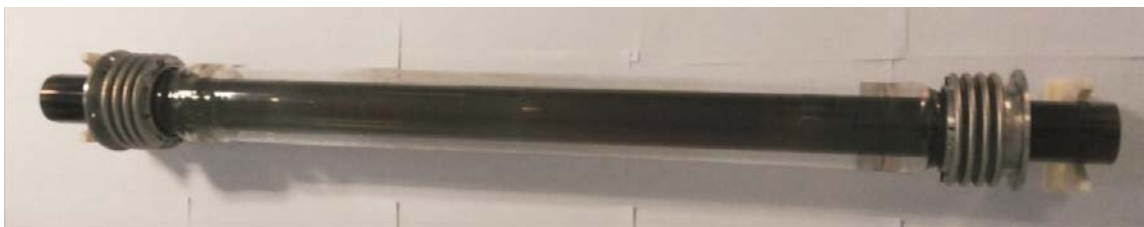
1 m long tube for solar thermal receiver
