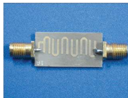
Band pass filter fabricated using indigenously developed MW substrates
