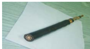
Sample cable of 50 mm 2 area and 33.80 mm dia
