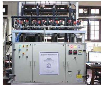
Adsorption system based solar cooling-cum-potable water production developed by IISc, Bangalore.
