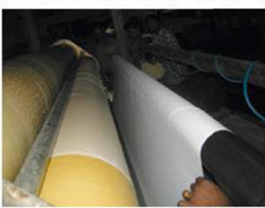
Dyeing of cotton fabric using pink dyes using industrial jigger machine
