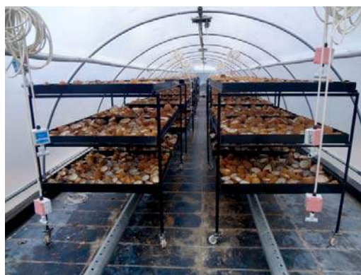
Solar tunnel dryer integrated with biomass hot air generation system
