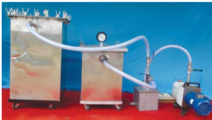
Mechanized sugarcane sett/bud treatment-prototype model
