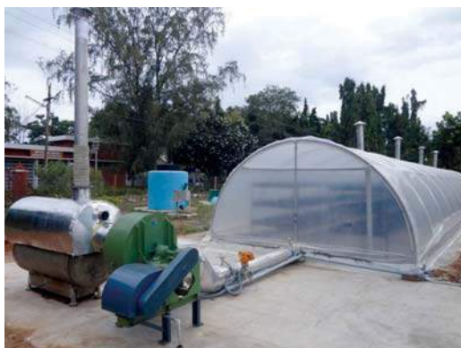
Solar tunnel dryer integrated with biomass hot air generation system
