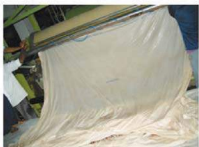
Dyeing of cotton fabric using pink dyes using industrial jigger machine
