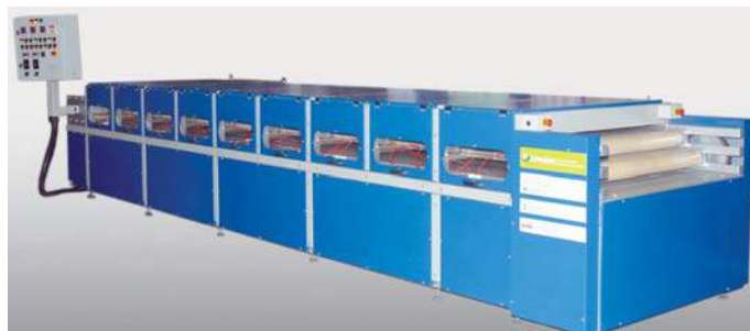
Atmospheric pressure plasma system for angora wool treatment
