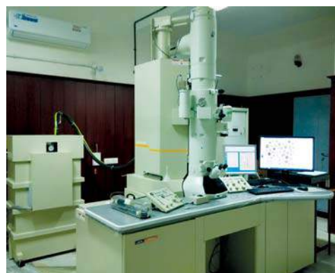
200 KeV Transmission Electron Microscope at the SAIF, Kochi
