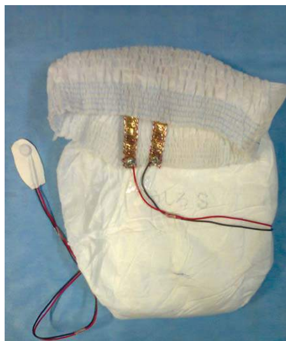
Leak Sensor embedded in a Diaper
