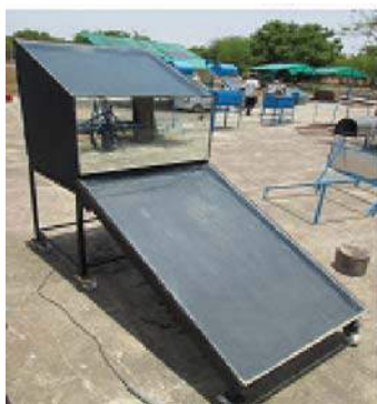
Solar crop dryer developed by CAZRI, Jodhpur
